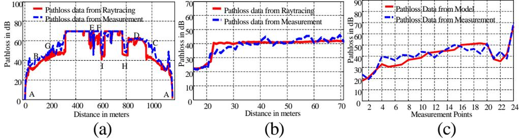
**Figure 4.** This figure compares the results of the measurements with the results obtained from the propagation model. The indices (a), (b) and (c) depict the comparison results for the campus map, an intersection in Philadelphia and interior of a building respectively as shown in the Figure 2
