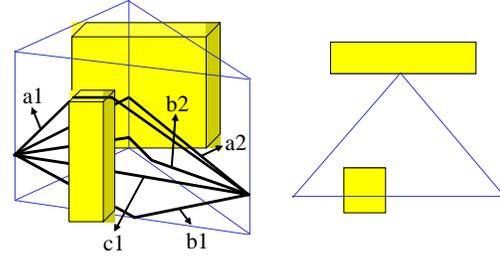
**Figure 1. Left: Two vertical plane paths and 5 ray paths. Right: a top-view of the scene on the left.**
