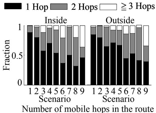
**Figure 6: Number of mobile hops in the route. There is always one mobile hop to a mobile end host. If there is more than one mobile hop, then the route contains a mobile-to-mobile link.**
