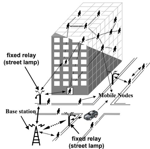
Figure 1: A conceptual visualization of mesh networks.
