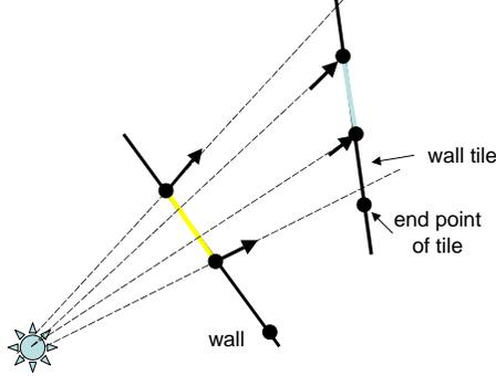
Figure 1: Beam Tracing. Suppose that the (yellow) tile on the lower left has been determined to have been hit by the beam. In particular, this beam hits the end points such that the reflected rays are as shown. From these rays, the virtual source, shown in the lower right is found. The angle at which the beam hits the end points of the (blue) tile in the upper right is found as shown. These rays as translated into reflected rays according to Snell’s Law and the process continues.
